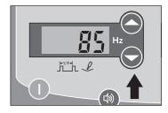
Upon completion of operation, confirm that the LCD screens are off and unplug the probe cords from the unit. If the unit is not to be used for an extended period, store it with the batteries removed.
